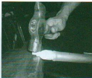
Fig 13. Forge the tip on the anvil's edge to clamp the rod.
