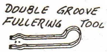
DOUBLE GROOVE FULLERING TOOL 1/4" ROUND WELDED 2" O.C. ON OUTSIDE FIG 2
