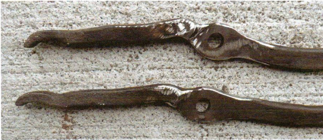
Figure 2: Tongs separated, sharp edges removed and trimmed for weight.
