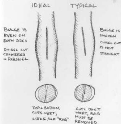
5. *Common slitting problems... always remove any steel "rag" left in the center of the hole.*
