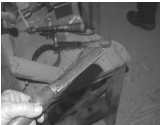
Broom making tool used to press (hammer) the wire, used to do the initial attachment of the corn to the handle, down tight onto the corn.
