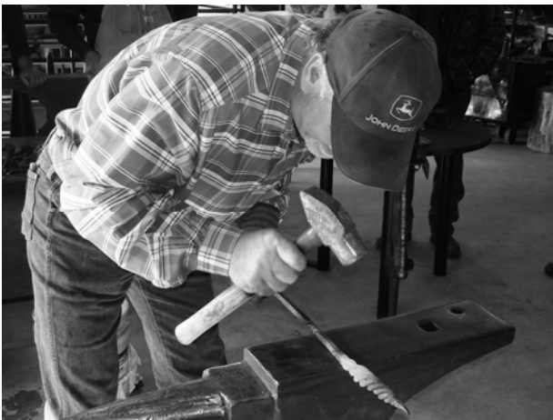
Dorvan working on a forge weld on his steak turner.
