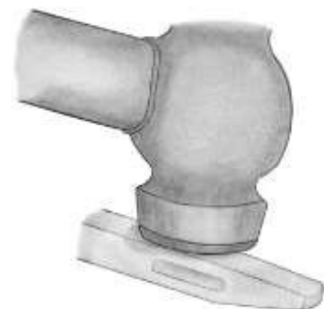
Keep the hammer centered over the back of the fullered bar, as shown above and in the next two illustrations.
